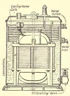
Fig. 246.—The water-cooled transformer.
